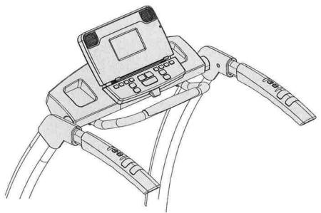
Contact Heart Rate Sensors are built into the stationary hand grips of the treadmill to monitor your heart rate during exercise. To use, grasp the sensors with a comfortable grip, with the palms of your hands placed over the sensors. If the sensors are having difficulty picking up your heart rate you may consider using aloe or a moisturizer on your hands or you can warm up as you exercise to increase the moisture in your hands. Dry hands do not transfer your pulse as effectively as moist hands.
