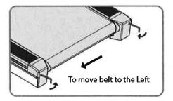
If you find that the belt comes out of alignment easily when you start using it, the belt is most likely too loose. A loose belt will slip across the rollers easily to the side your body favours. If this is the case, please follow belt tensioning procedure below after aligning belt.
