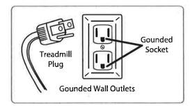
**Danger:** Improper connection of the equipment grounding conductor can result in the risk of electric shock. Check with a qualified electrician or service person if you are in doubt as to whether the product is properly grounded. Do not modify the plug provided with the product. If it will not fit in the outlet, have the proper outlet installed by a qualified electrician.
