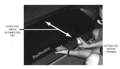
The silicone icon shown below will display every 100 hours of use, regardless of whether the treadmill has been lubricated or not. It is simply a background reminder to ensure the owner does not forget this essential maintenance. Remember however, the periodic maintenance schedule is every 40 hours or once per month. The icon will turn off after 5 minutes, or press "SPEED DOWN" and "START" buttons simultaneously until icon disappears.
