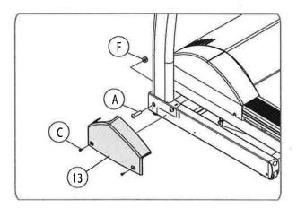
C. Attach the left (13) and right (14) base covers using Phillips screwdriver and 2 machine screws on each side. The 4 base cover attaching screws are located in the hardware bag.
